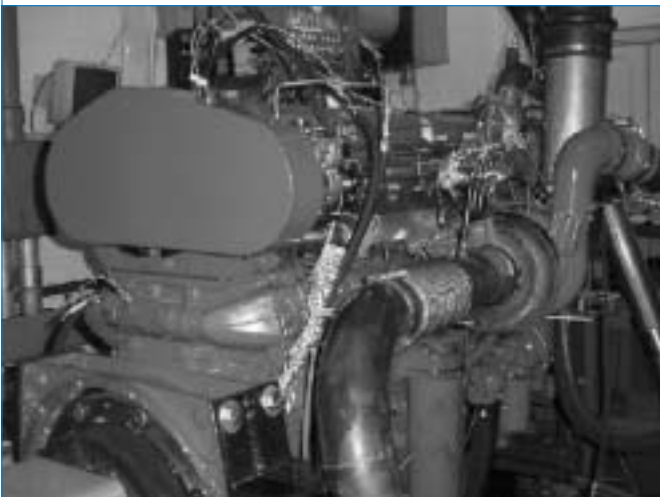
Figure 8. The heavy-duty NO x engine is shown in the test cell.
