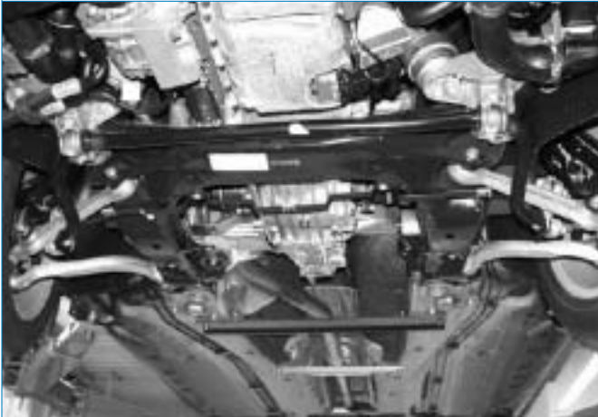
Figure 3. The passenger car underbody accommodates the ECS components.
