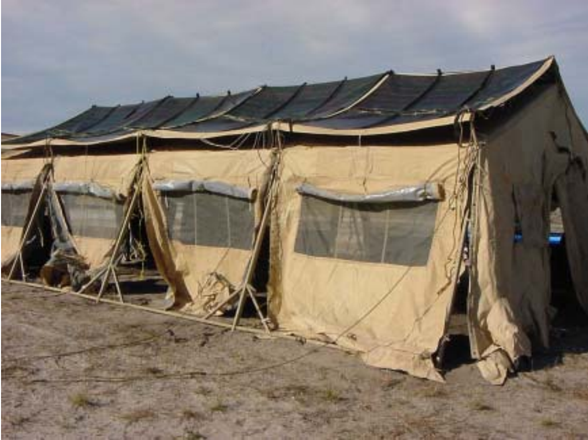
Figure 3.4: Power Flex™ modules on tent during tent deployment
