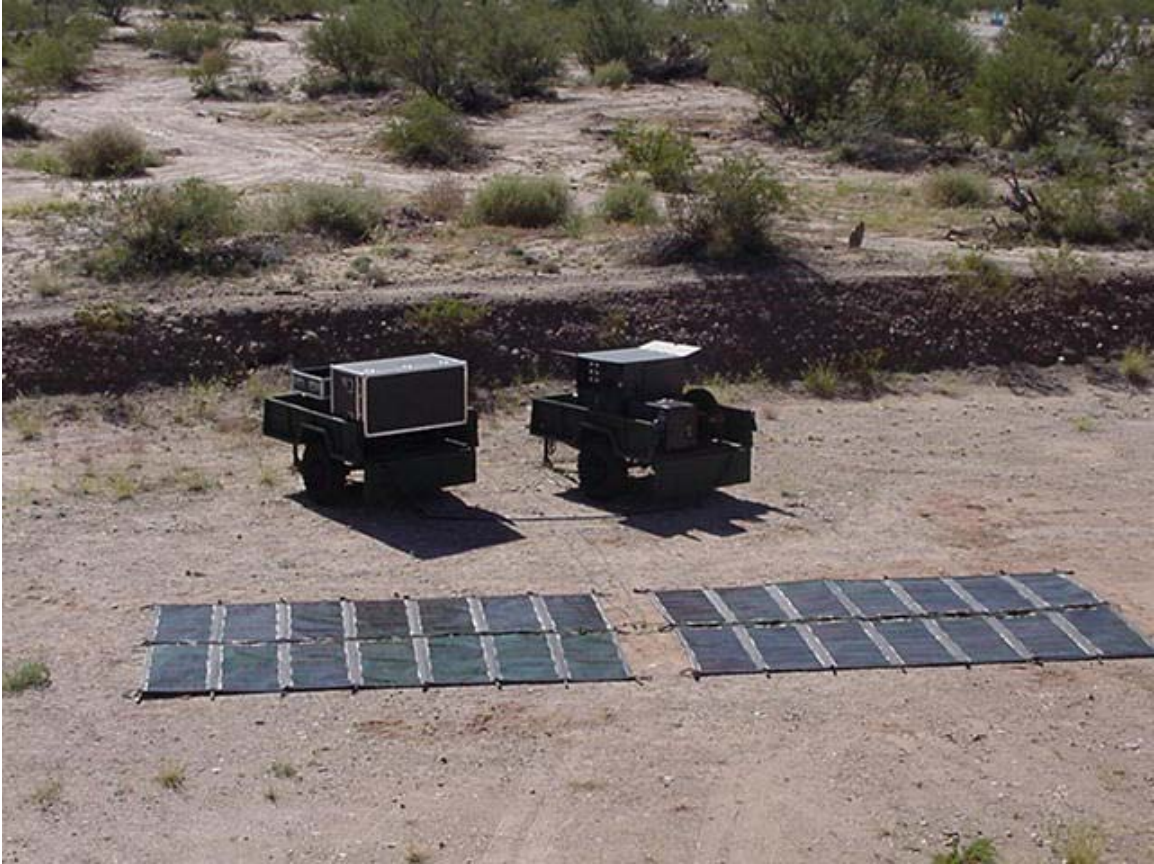
Figure 3.3: Power Flex™ modules on ground
