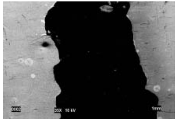
Figure 1.13b: Scratch test exhibiting poor adhesion
