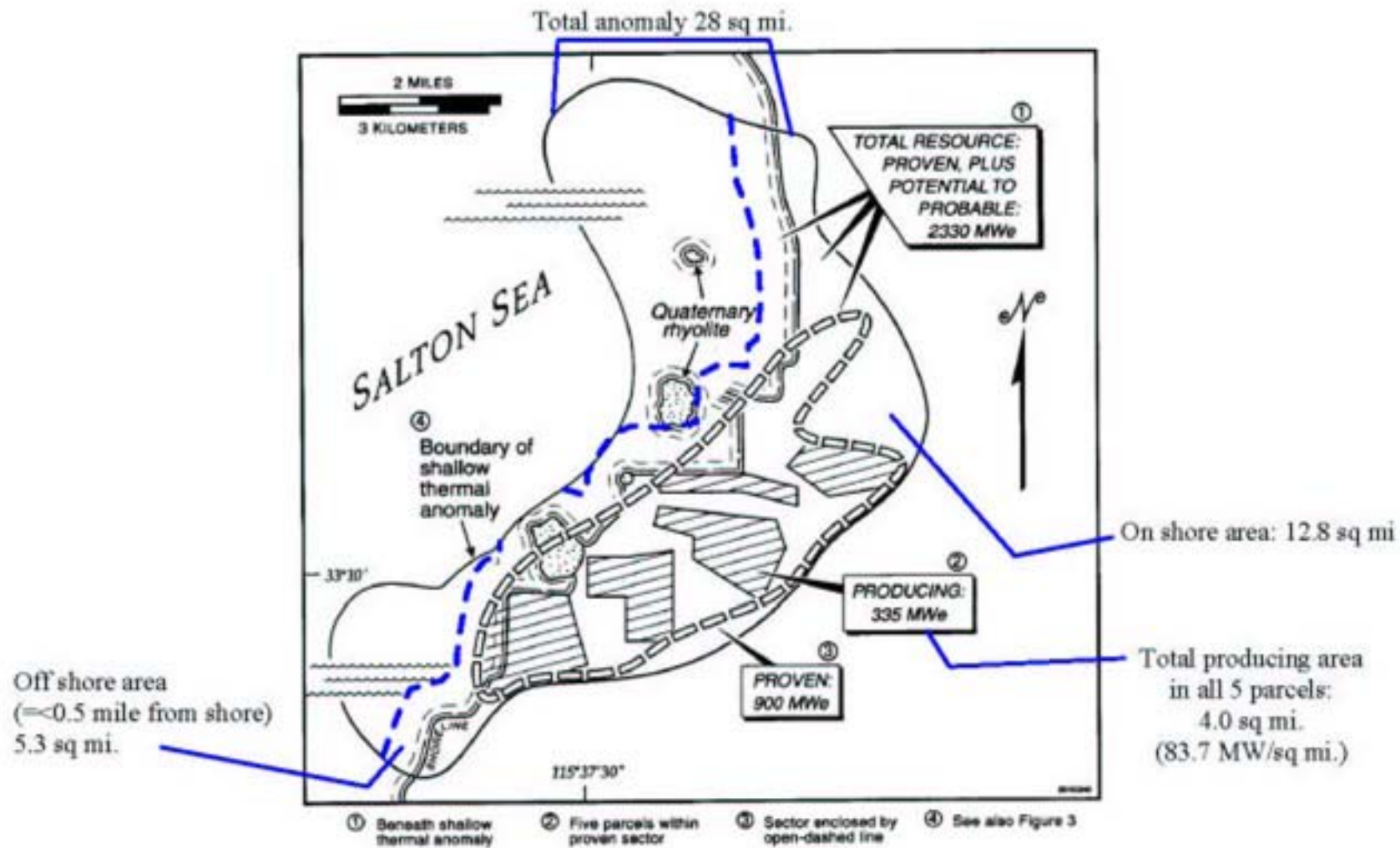
Figure 6. Map showing estimated ultimate conventional resource potential for the Salton Sea geothermal field as of July 2002.
