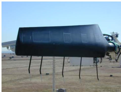
Figure 14: Leading edge sensor booms (NREL)
