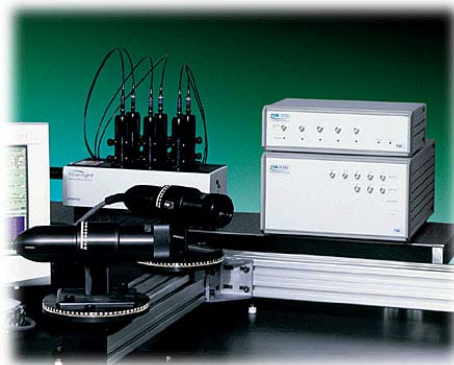
Figure 18: Laser Doppler velocimetry system
