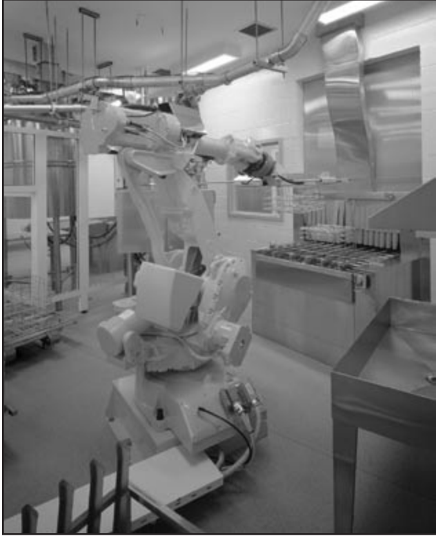
Figure 3. Robotics used in cage washing operation
