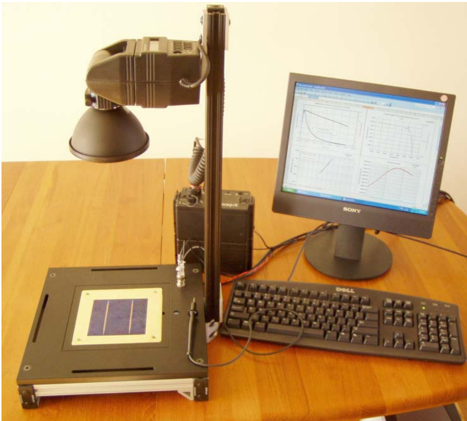
Fig. 39. The current version of the Suns-V oc instrument. The large chuck can accommodate 6-inch wafers. The stage is magnetic, so that it can be used with magnetic-base probes.
