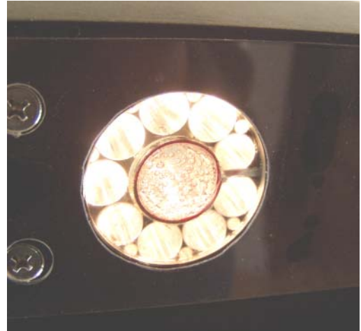
Fig. 14. This sample head is optimized for in-line measurements of wafers or flat surfaces of uniform blocks. The illuminated area is large, to enable high sensitivity for measuring unpassivated wafers just entering the process line, and giving very one-dimensional results on phosphorus-diffused wafers.
