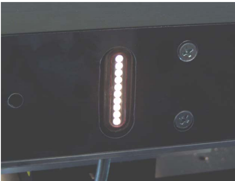
Fig. 8. A detail of the block scanner, the sense head. This spot size is about 3 mm wide, and 30 mm high giving high resolution when stepped in the long (growth) axis of the block. The result is averaged over 30 mm in the axis perpendicular to the growth direction. The total illuminated area is large enough to give very good signal to noise.
