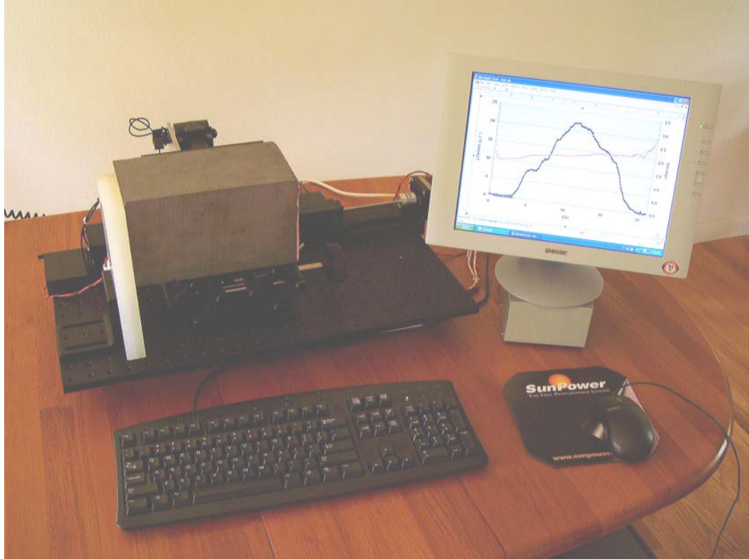
Fig. 7. This instrument performs line scans down the length of a Multi-crystalline silicon block. The sample head, (behind the block) is run along a computer-controlled stage.
