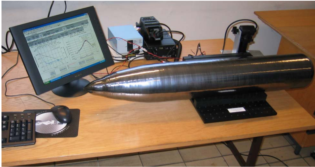
Fig. 13. An instrument that was optimized for measurements on as-grown boules of high-lifetime float-zone silicon. (Photograph courtesy of Jan Vedde, Topsil A/S).
