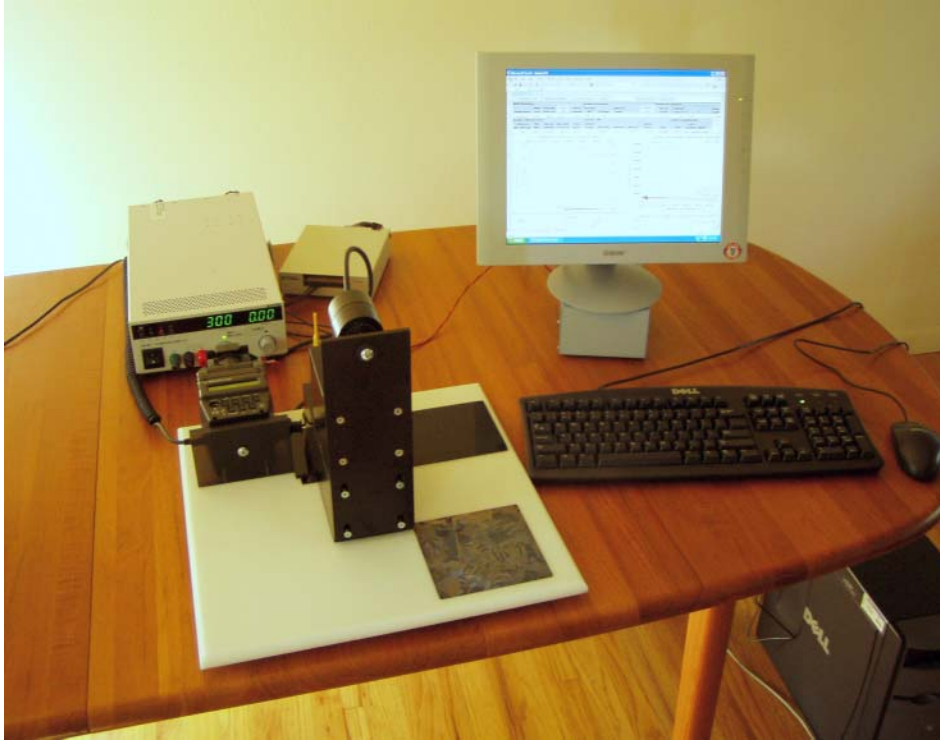
Fig. 21. A sample head that can be mounted in a production line to measure every wafer. The measurement area is an 8-cm diameter.
