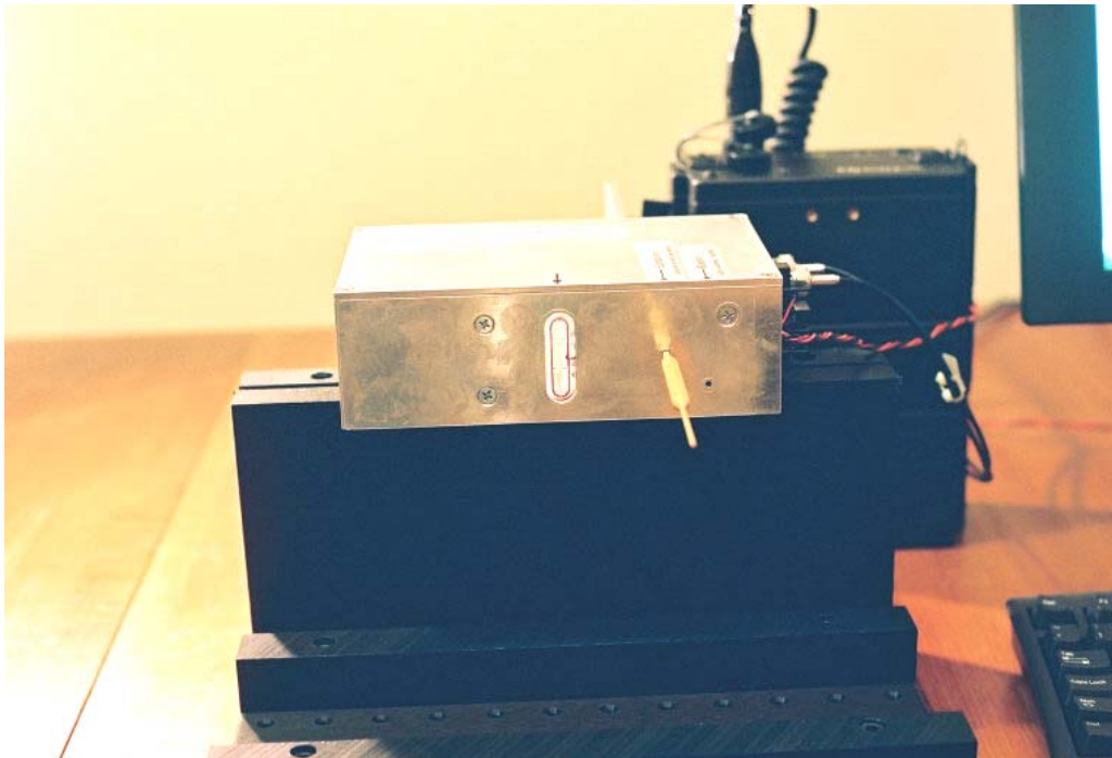
Fig. 5. The shape of the sensor is optimized for flexible measurements of blocks. The relatively large area gives a large photoconductance signal, and insures that the device physics of the analysis is primarily one-dimensional. The long slender shape of the sensor permits measurements on cylindrical shapes, since the sensor and illumination is nearly planar to the sensed portion of a cylindrical ingot when used in the geometry shown in Fig. 4.
