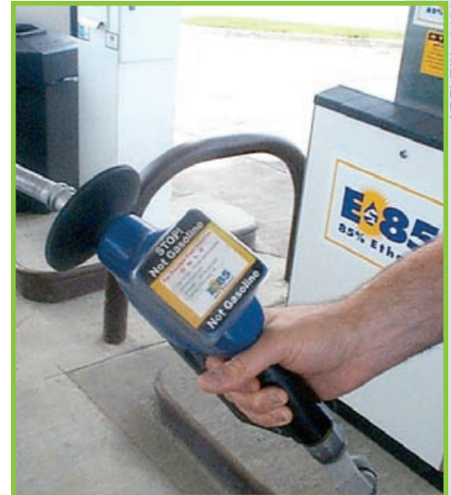
E85 pumps look much like gasoline dispensers, but their parts must be made of stainless steel to prevent corrosion.
