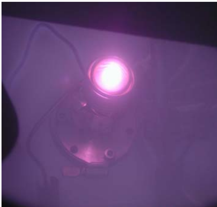
Figure 50 : PACE source with plasma operating in three-stage CIGS co-evaporation chamber.
