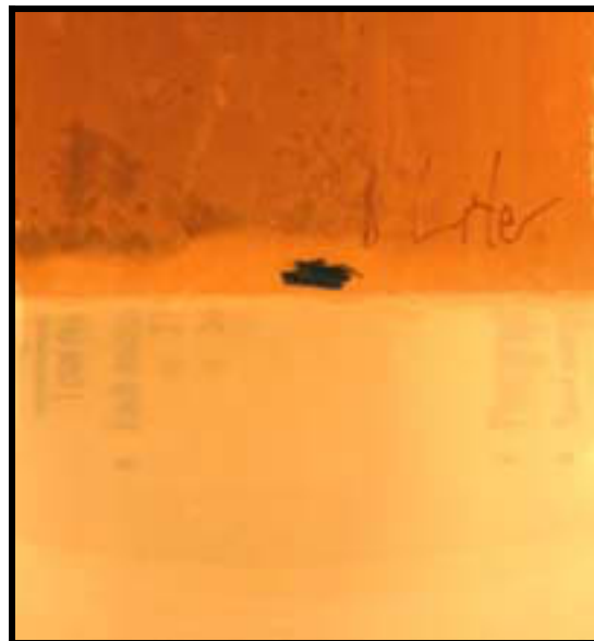
Figure 4. Stage 2 microcosm fuel-water interface 5-weeks post-challenge.
