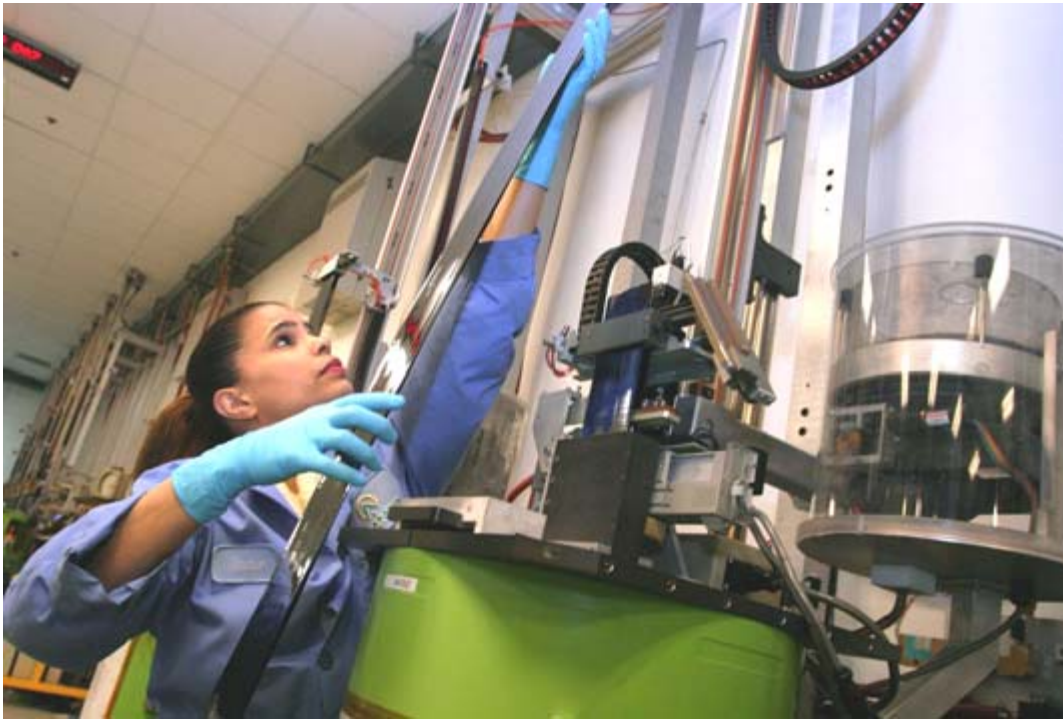
Figure 10 - Production operator removing two Gemini ribbon strips simultaneously.
