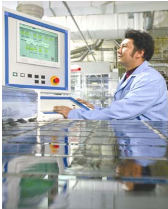
Figure 27 - Diffusant glass removal station. Rows of cleaned, diffused cell blanks can be seen emerging from the machine.
