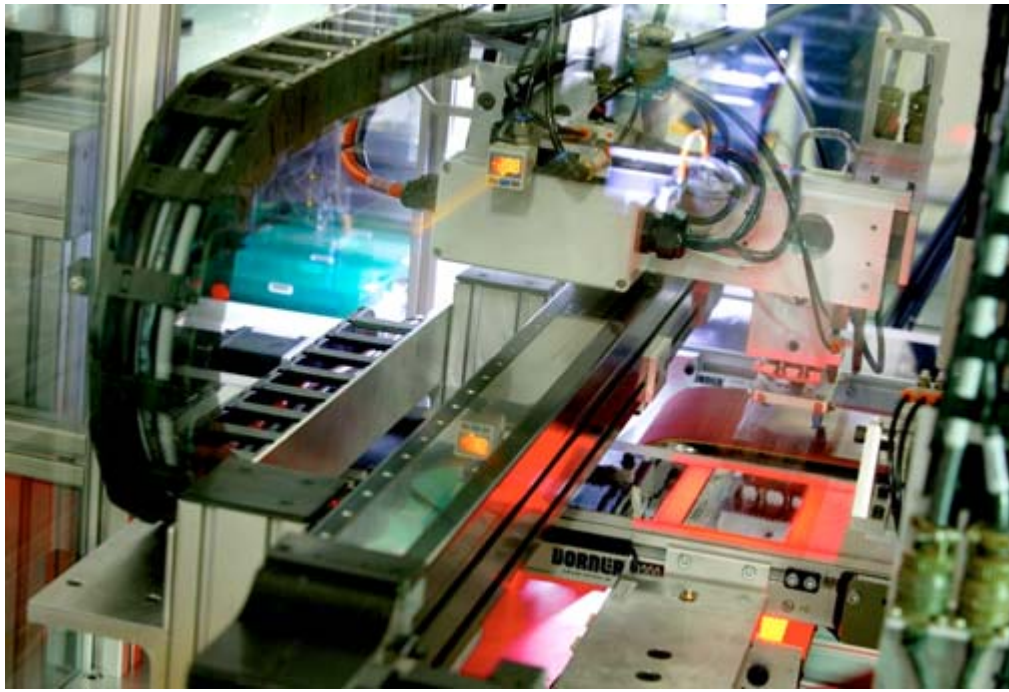
Figure 28 - Robotic loading onto the silicon nitride deposition machine.
