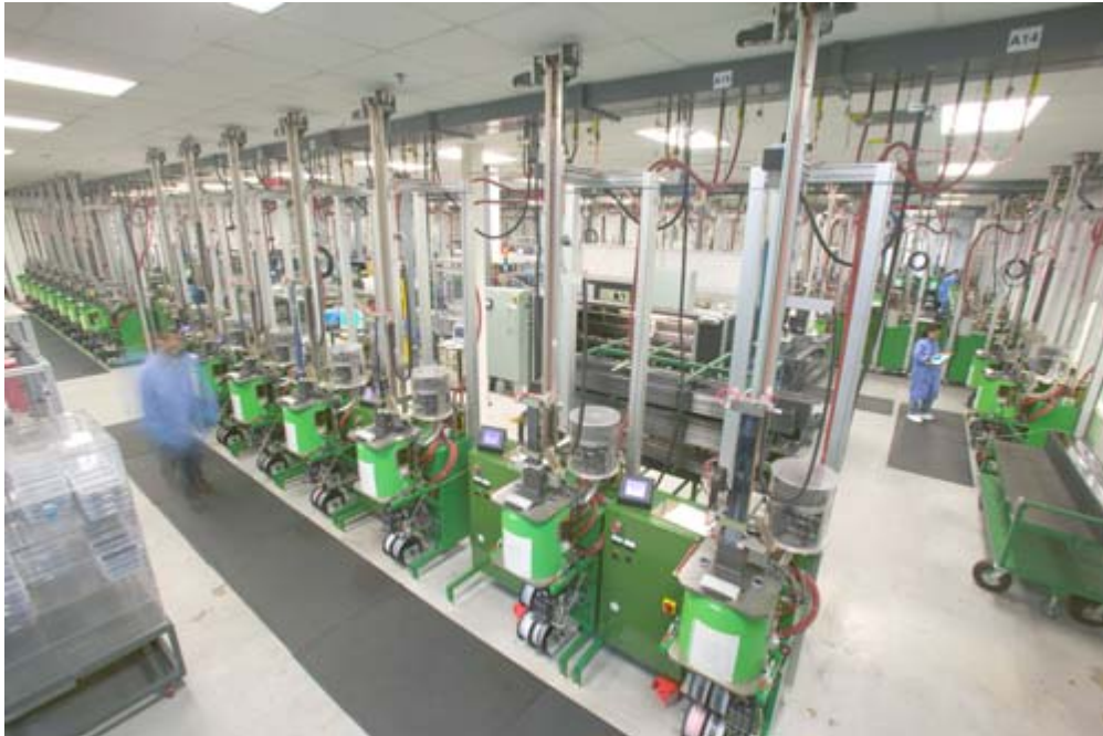
Figure 18 – Aerial view of the production crystal growth area with all Gemini furnaces.
