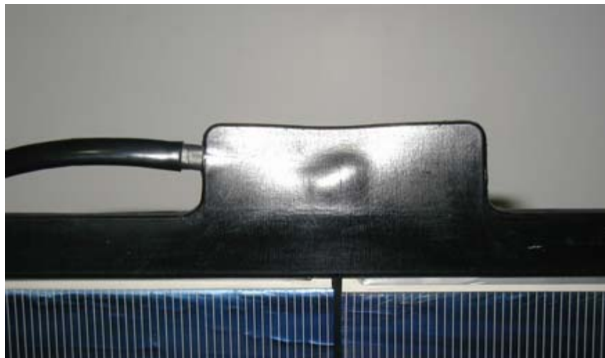
Figure 44 – Top front of a monolithic module showing the region where the leads emerge from the module.
