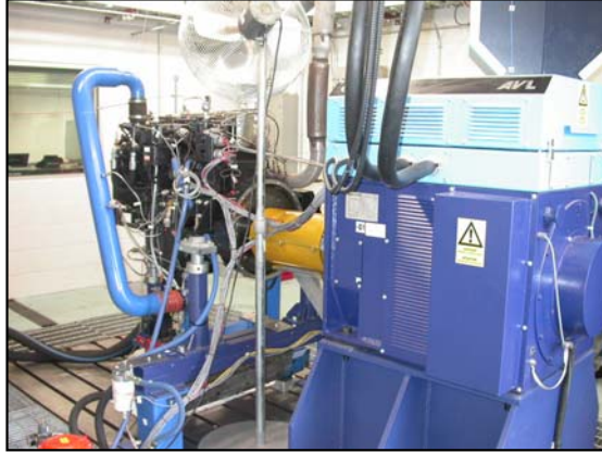
Figure 3: Engine test cell with B Gas Plus engine installed and connected to the Dynamometer.
