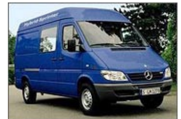
The Sprinter van is a prototype plug-in hybrid vehicle developed by EPRI and DaimlerChrysler.
