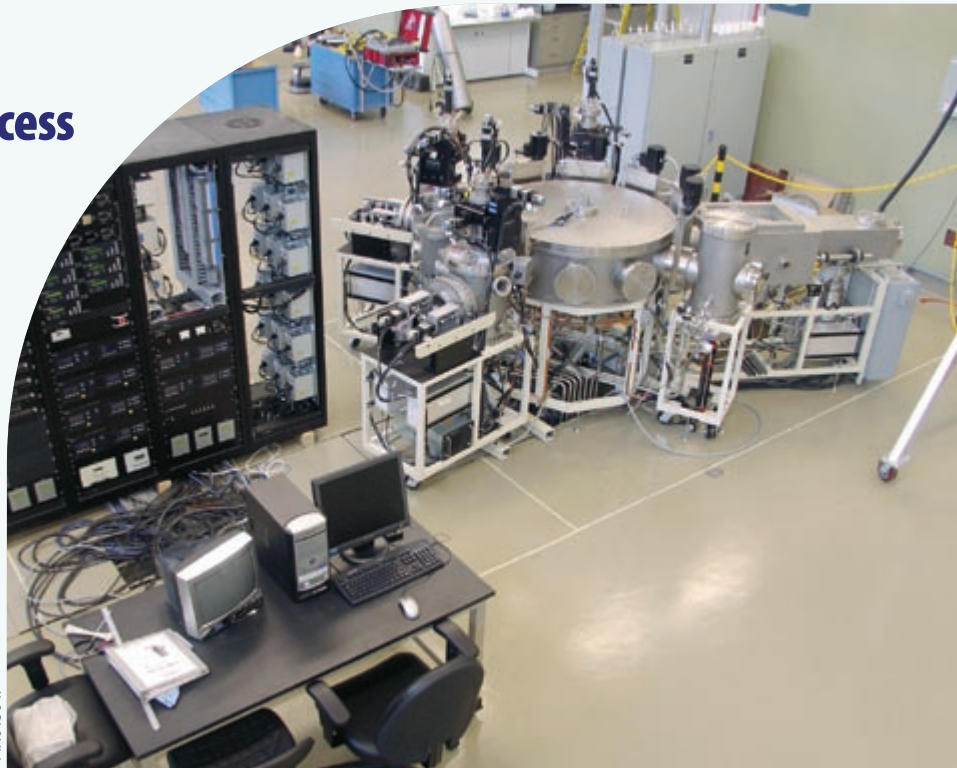
The silicon cluster tool, which allows for robotic manipulation of silicon solar cells in a vacuum environment, was the first addition to the new PDIL.
