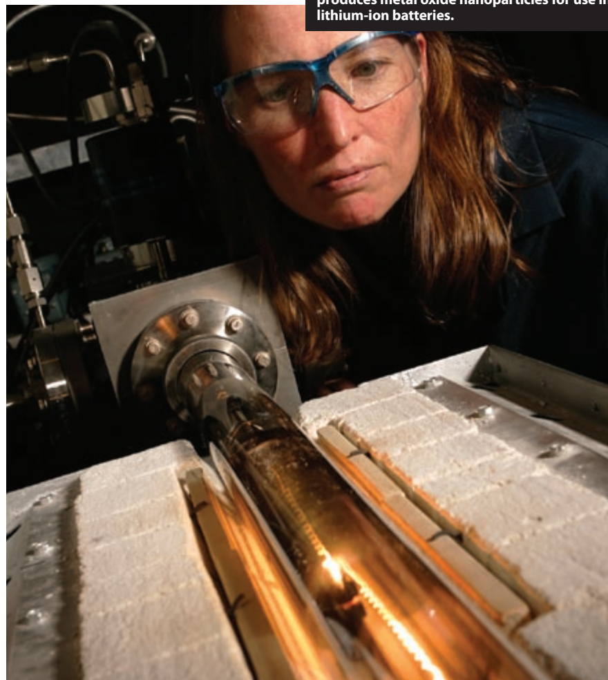
NREL Scientist Anne Dillon examines the hot-wire chemical deposition system, which produces metal oxide nanoparticles for use in lithium-ion batteries.
