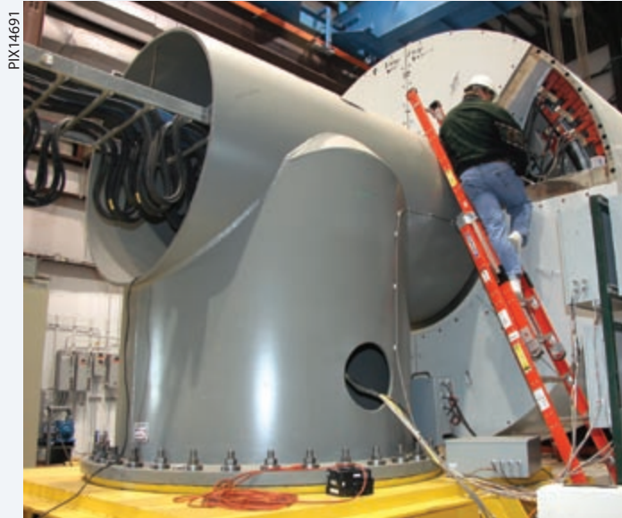
NREL worked with Northern Power Systems to develop a 1.5-megawatt direct-drive generator for wind turbines, shown here during testing at NREL's National Wind Technology Center.
