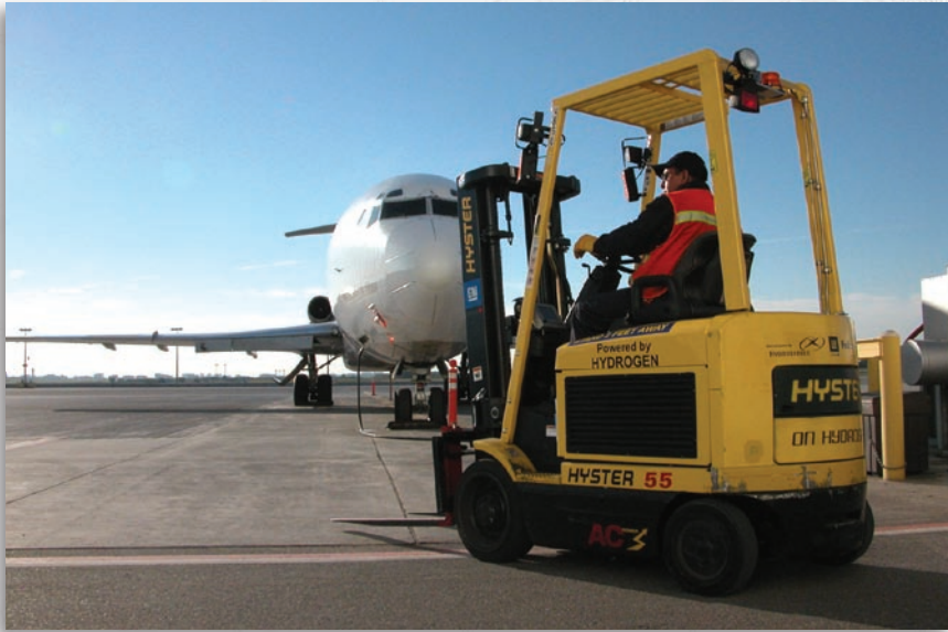
PEM fuel cell forklifts such as this one can increase productivity and can be cost competitive on a lifecycle bases for continuous use operations.
