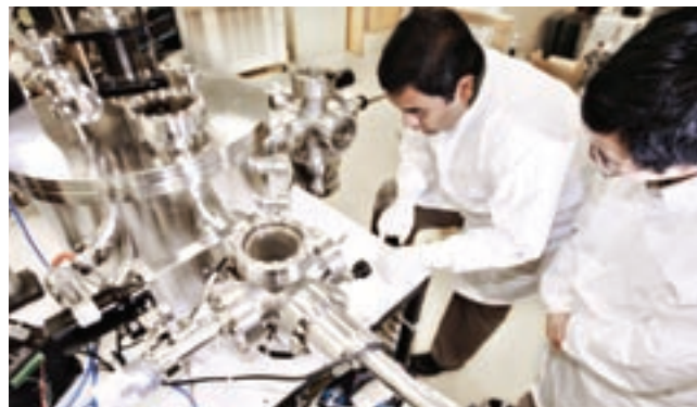
Researchers from Planar Energy Devices, Inc., insert a sample into the vacuum chamber of the company's thin-film deposition system.
