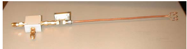
Figure 12. Photo of a branch of the RCPCD measurement circuit showing (from left to right) the directional coupler, shielded capacitor, length of coaxial cable, and coil antenna.
