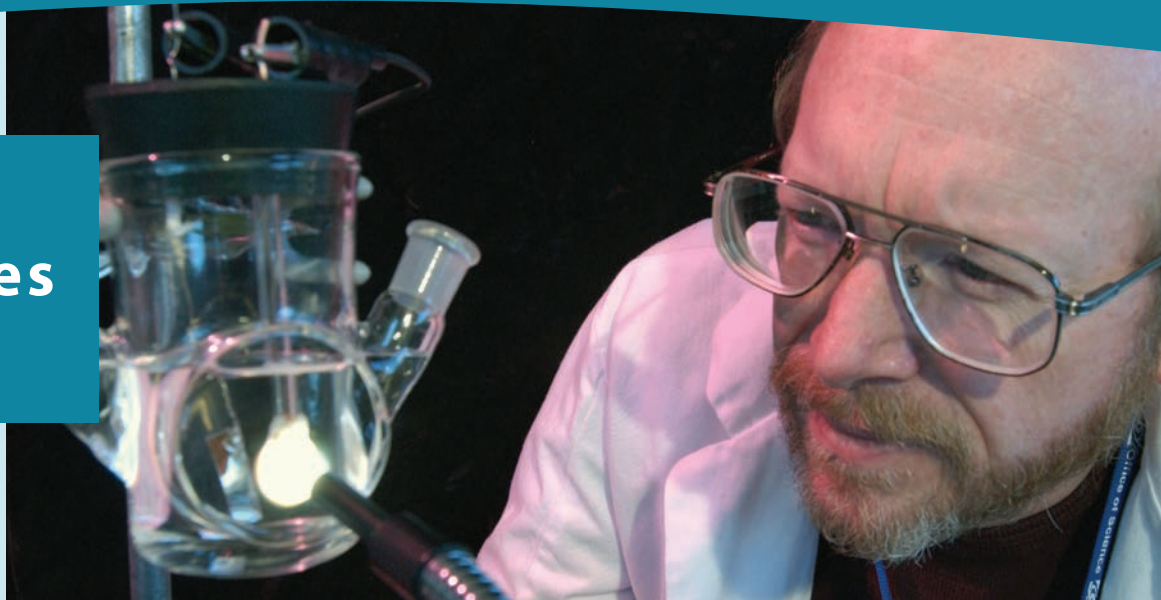
Photoelectrochemical water splitting: Using a photovoltaic cell/electrolyzer submerged in an alkaline aqueous solution to produce hydrogen. Photo by Richard Peterson, NREL/PIX12958
