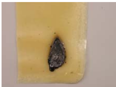
Figure 64. Flame impingement test: Compound X122-47-1.
