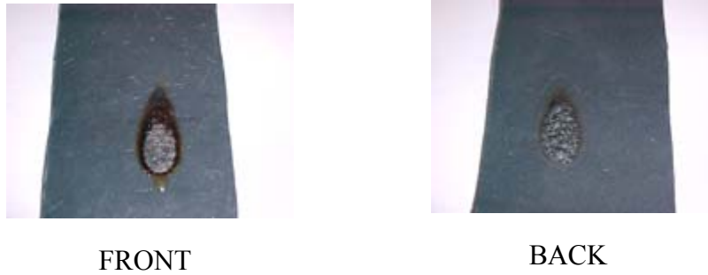
Figure 9. Flame-impinged samples of non-halogenated FR formulation.
