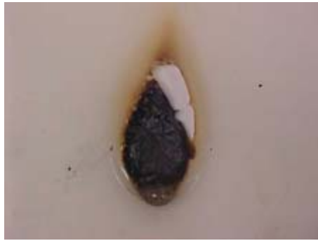
Figure 60. Flame impingement test: Compound A.
