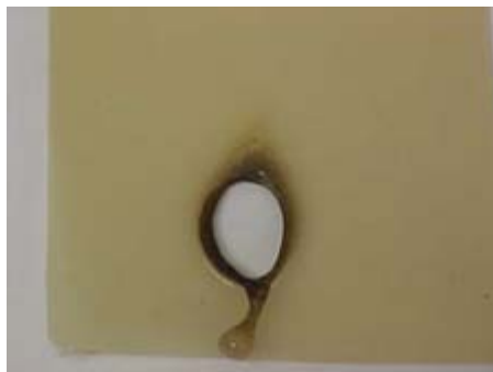
Figure 63. Flame impingement test: Compound EV4.
