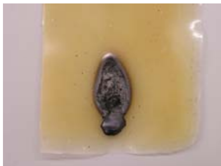
Figure 65. Flame impingement test: Compound X122-47-2.
