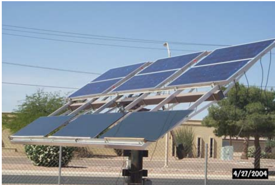
Figure 50. 2-axis tracker at ASU-PTL bearing SFC- and FR-laminated modules (top six modules).
