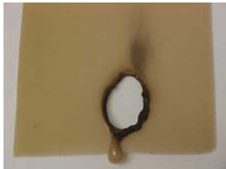
Figure 62. Flame impingement test: Compound EV2.
