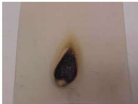
Figure 61. Flame impingement test: Compound B.
