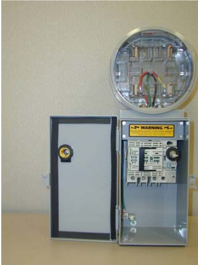
Fig. 2-2. The interior of the meter interconnect's custom enclosure houses the fused disconnect switch. An interior ground lug is provided and all live parts are fully protected from touch. A shaft into the body of the switch extends through the cover to the handle on the outside. A gasket seals the door against the box.
