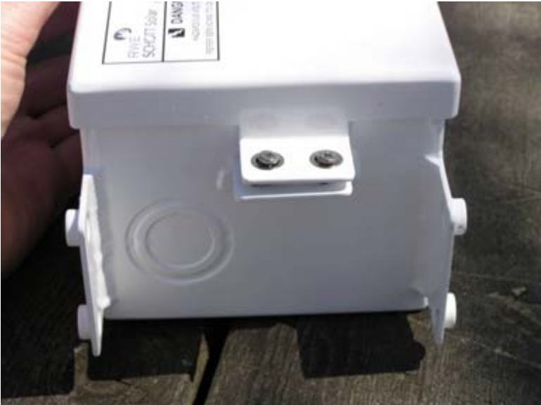
Fig. 7-3. Box lid secures to box base with two captive fasteners on tab. Mounting flanges contain pressed-in 1/4-20 nuts for simplified attachment to the company's PV array mounting hardware.
