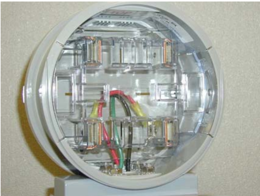
Fig. 2-7. The clear plastic shield prevents inadvertent contact with the factory wiring and sockets in the meter extender.
