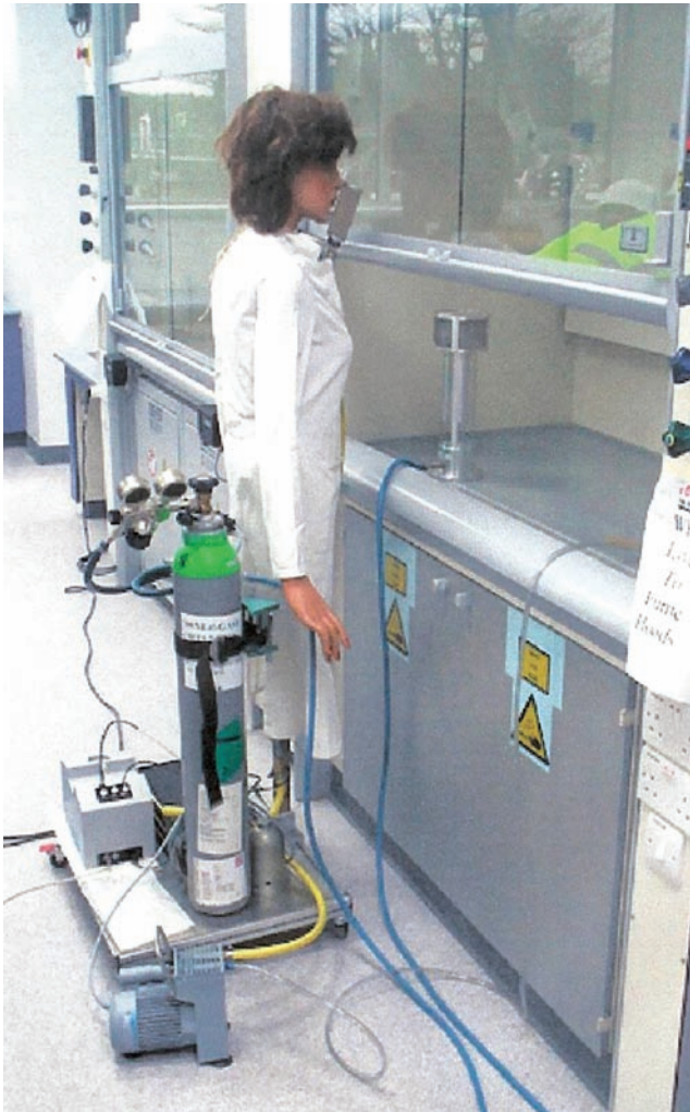
Figure 3. Mannequin simulates worker exposure during a tracer gas test.
