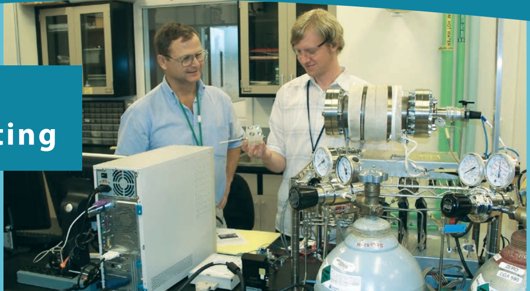
NREL researchers William Buttner and Matthew Post setting up a test for a commercially available hydrogen sensor. Because hydrogen is colorless and odorless, sensors are key safety elements of fueling stations and other hydrogen facilities. NREL/PIX 15977
