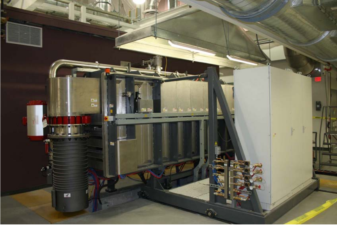
Figure 2.2. A GSE tool for roll-to-roll absorber (CIGS) deposition at the new manufacturing facility in Tucson.
