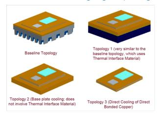
Developed basic framework for rapid assessment of interactions between thermal packaging topologies, materials, and thermal performance.
