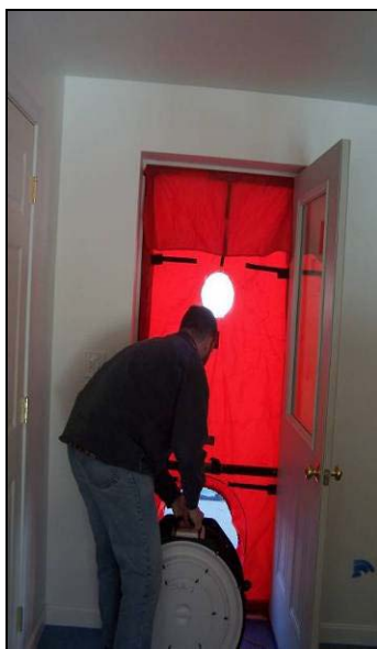
Figure 11. Blower door test setup
