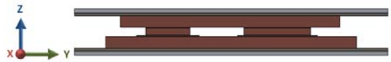
Figure 2. Double-sided package showing side view of IGBT and diode with a 50 mm by 30 mm heat exchanger base area.
