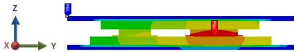
Figure 4. Sample of temperature distribution on ANSYS FEA model (coolant temperature 70°C, IGBT junction temperature 150°C, net effective UA applied to each side 10 W/K, IGBT heat flux 170.7 W/cm 2 , IGBT to diode loss ratio 3:1).
