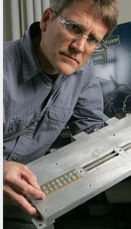
Ken Kelly holds a Semikron inverter that has channels built into it for liquid cooling of its power electronics.
