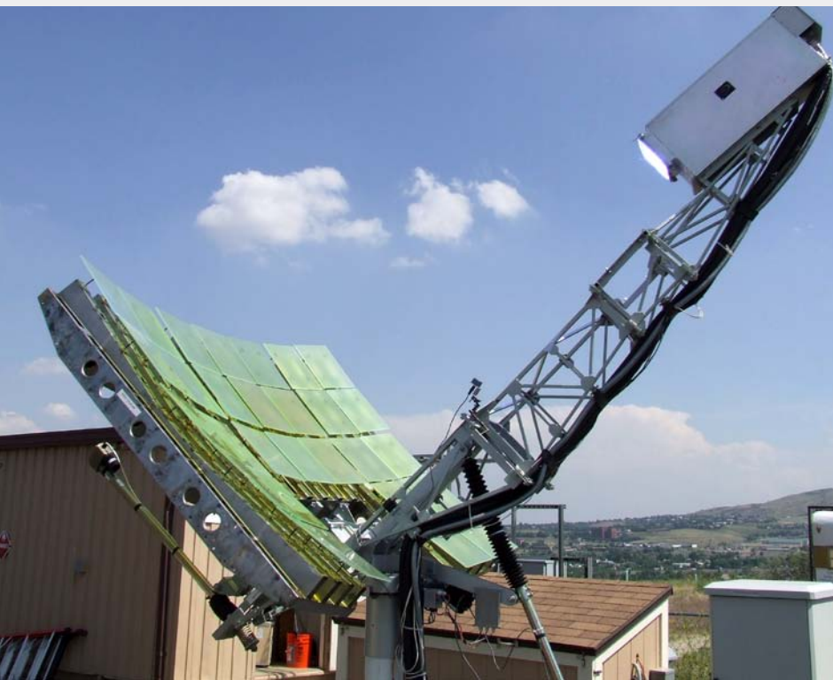
The Ultra-Accelerated Weathering System concentrates ultraviolet light on test samples while rejecting the solar wavelengths that would cause the samples to overheat.
