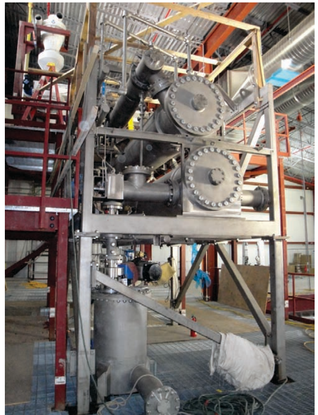
Figure 2. The one dry ton/d pretreatment reactor system consisting of four horizontal tube reactors of varying sizes and residence times (two large tubes and one smaller tube are visible) and a flash tank (bottom of picture). Feedstock is pneumatically conveyed from the basement to the cyclone (top left of picture), weighed, and then fed to the reactor's pressure feeder.
