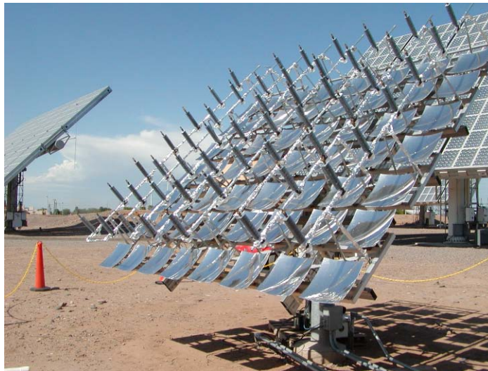
Fig. 3.1.5 A prototype of a high concentration module at the APS STAR facility using triple-junction concentrator solar cells. This system was the first grid-connected solar concentrator system using triple-junction cells.
