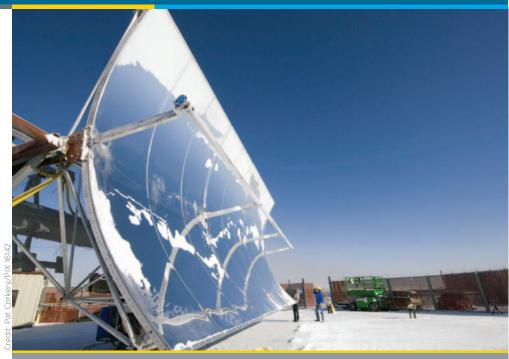
The SkyTrough solar concentrator was developed with highly-reflective, silver-metalized film that is lighter and less expensive than the glass mirrors that are traditionally used.
