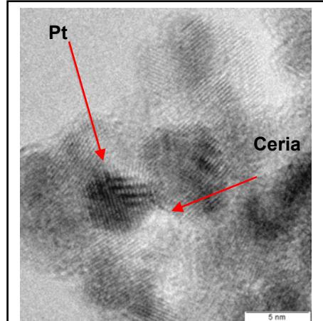
Using a core-shell material such as platinum-ceria for catalysis improves hydrogen spillover for storage
