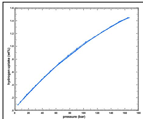
Hydrogen spillover capacity of a ruthenium-activated carbon material made with NREL's advanced synthesis process
