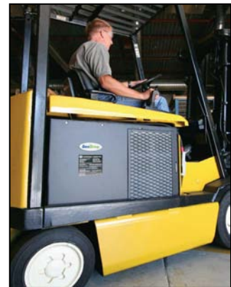
Figure 13: Plug Power GenDrive Fuel Cell Powered Forklift. Photo Courtesy of Plug Power.
