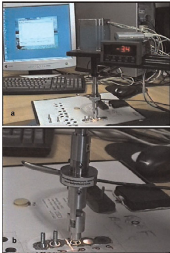
Figure 1. (a) System with stepper motor, 5:1 speed reducer, torque sensor, and universal coupler fitting that attaches to a Phillips flat-head screw epoxied to a cored Si cell; (b) close-up image showing details of torque sensor and coupling hardware
