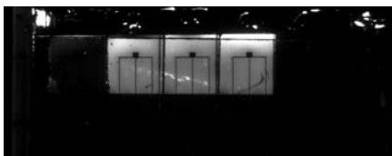
Fig. 10. PL image of M3147-12 re-fabricated with new layers of CdS, i-ZnO, ZnO:Al and Ni/Al grids.
