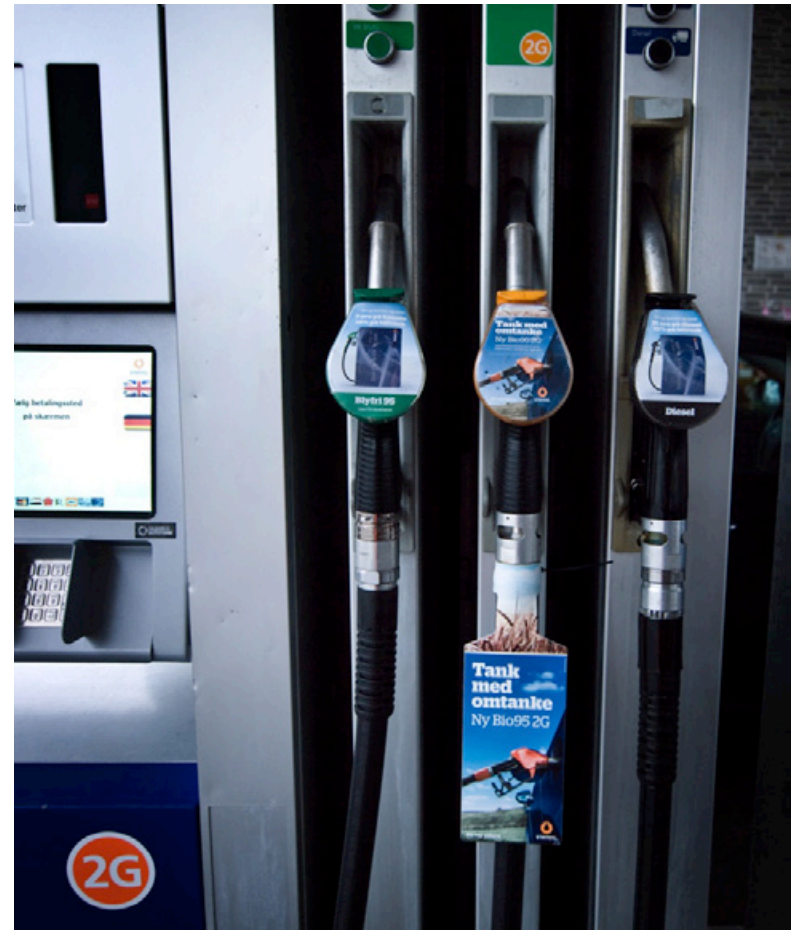
Danish fueling station pump dispensing E5 gasoline-ethanol blend containing wheat straw-derived cellulosic ethanol
