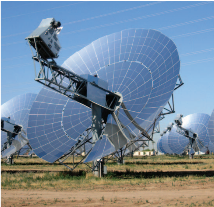
SunCatcher CSP dishes at the Maricopa Solar Power Plant in Peoria, Arizona, focus sunlight onto a Stirling engine to convert solar thermal energy into grid-quality electricity. The SunCatcher was designed and developed in the United States through a public-private partnership with DOE's Solar Program. Photo by David Hicks, NREL/PIX 18380
