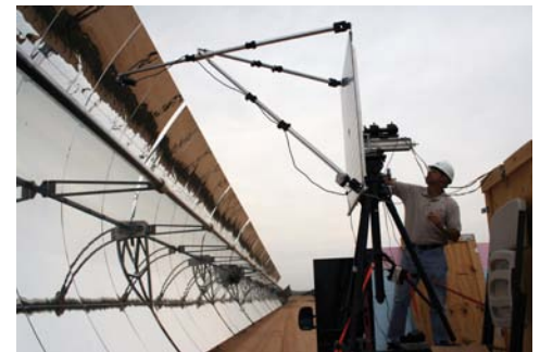
The National Renewable Energy Laboratory's (NREL) Video Scanning Hartmann Optical Test (VSHOT) laser scanning system determines the accuracy of concentrator mirror structures and is used in both a laboratory setting and in the field. Photo by Alison Gray, NREL/PIX 16739
