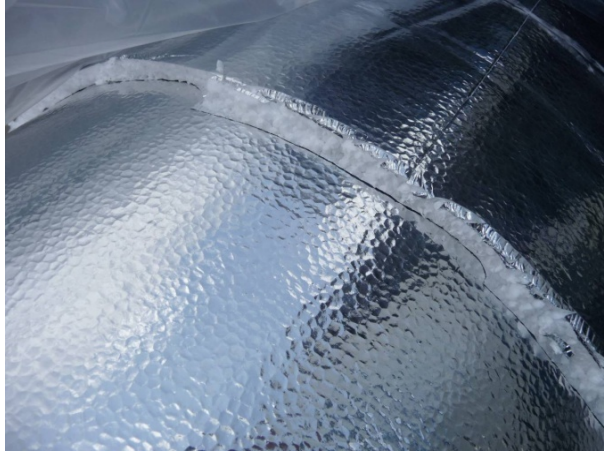
Figure 42. 3/8-in. beadboard insulation with foil face on one side and plastic film on the other.
