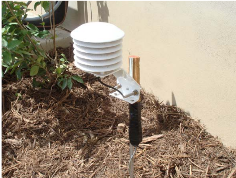
Figure 2. Outdoor temperature and RH sensor mounted far enough from the home so it will not be influenced by it
