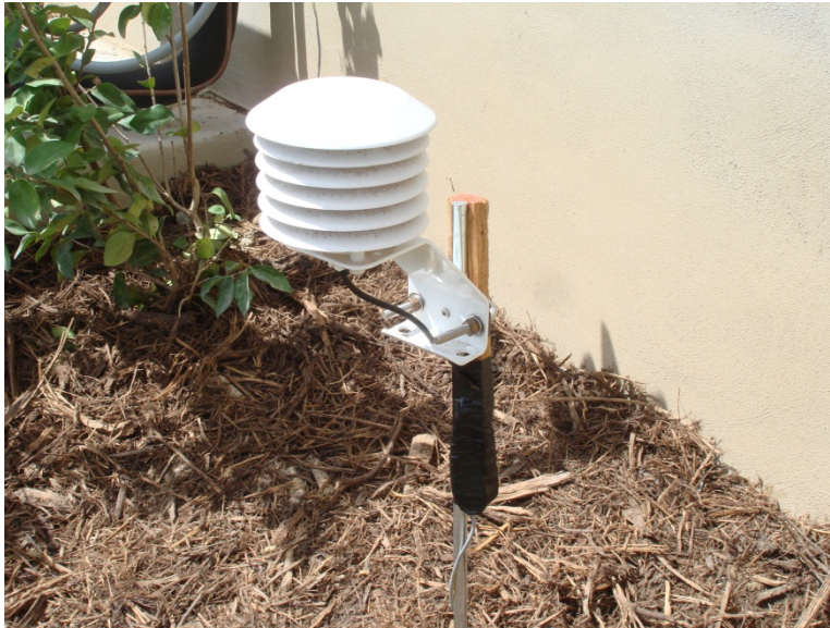
Figure 26. Location #5; outdoor temperature and humidity measurement
