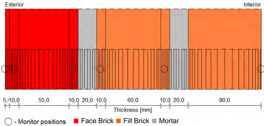
Figure 7. WUFI model of existing original building masonry wall assembly (solid brick wythes)
