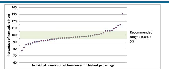
Figure 22. Measured fire rate as a percentage of nameplate input
