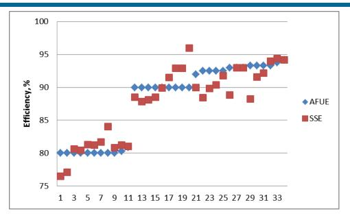
Figure 8. Label AFUE versus test-in steady state efficiency
