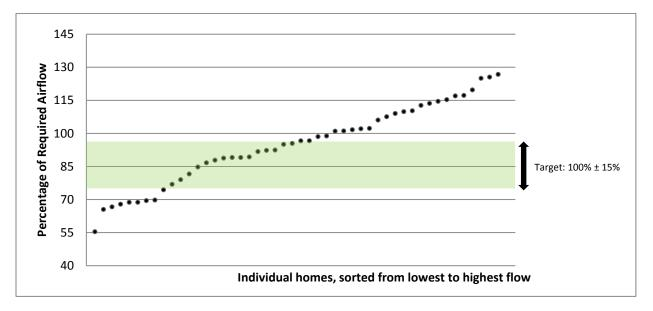
Figure 19. Percentage of required airflow across heat exchanger as measured in the home
