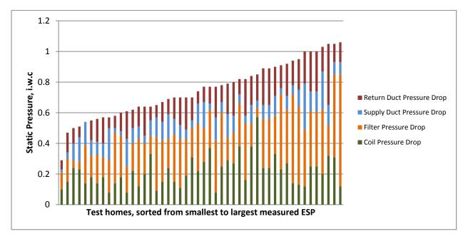
Figure 5. Recorded static pressure drop, by component
