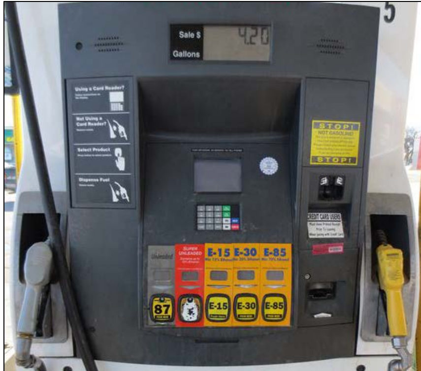
Figure 6. Station #17 offered E15 from same nozzle as higher ethanol blends
