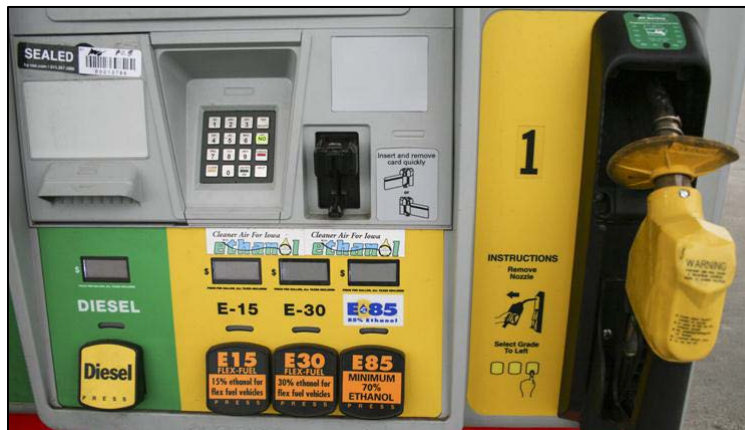
Figure 4. Station #1 offered E15 from same nozzle as higher ethanol blends
