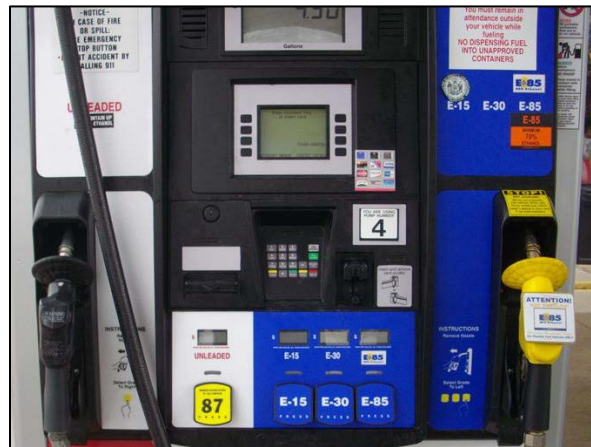
Figure 5. Station #2 offered E15 from same nozzle as higher ethanol blends
