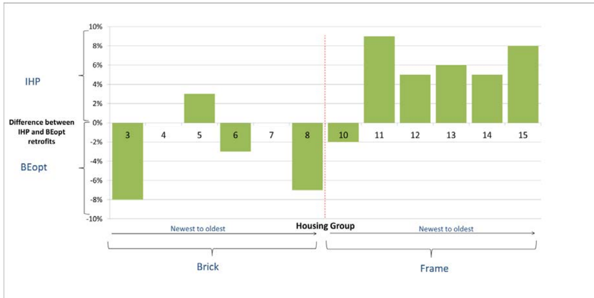
Figure 5. Modeled EUI reduction differences between IHP measures and BEopt-recommended measures
