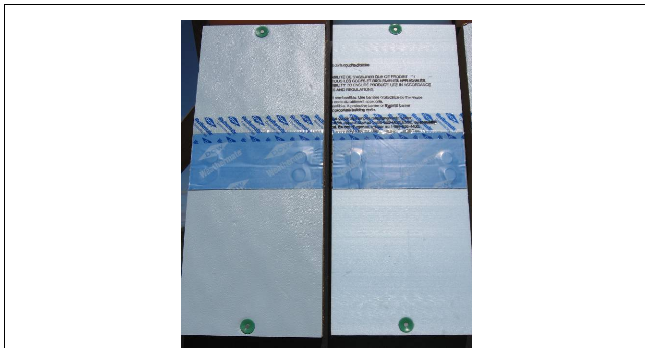
Figure 33. Dow Weathermate butyl with termination tape on ffPIC (left) and XPS (right)
