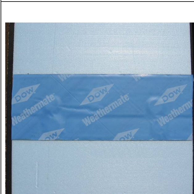
Figure 45. Dow Weathermate butyl on XPS—large sample
