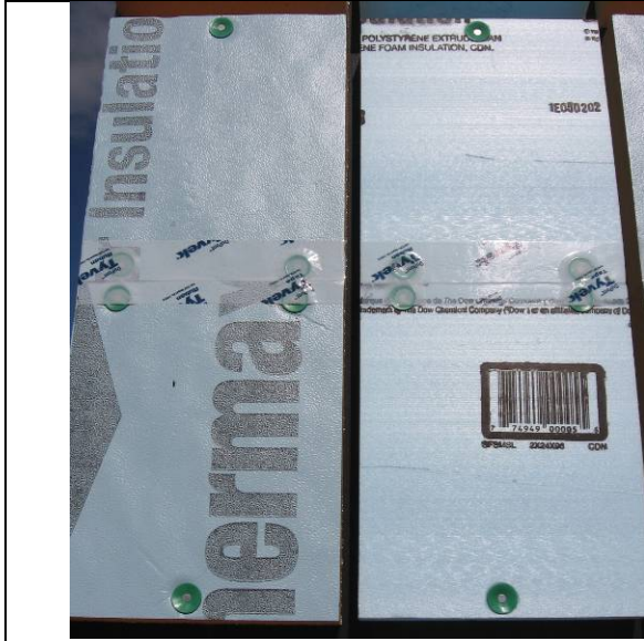
Figure 27. DuPont Tyvek tape on ffPIC (left) and XPS (right)
