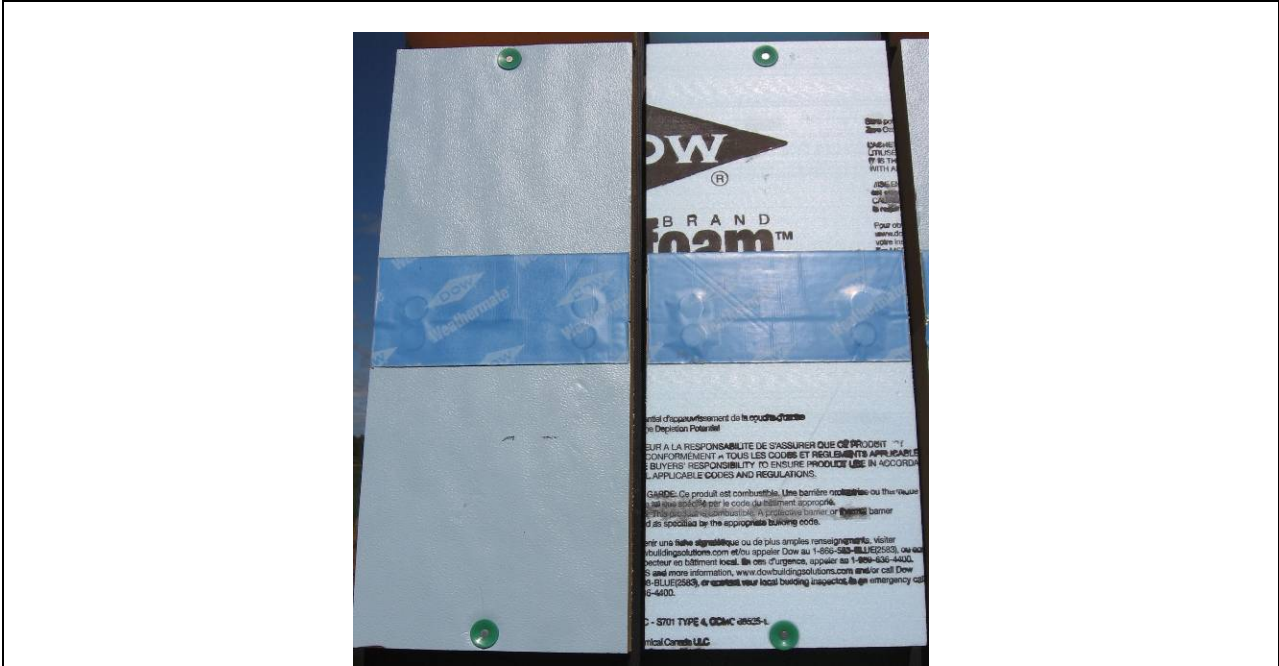
Figure 35. Dow Weathermate butyl on ffpic (left) and XPS (right)
