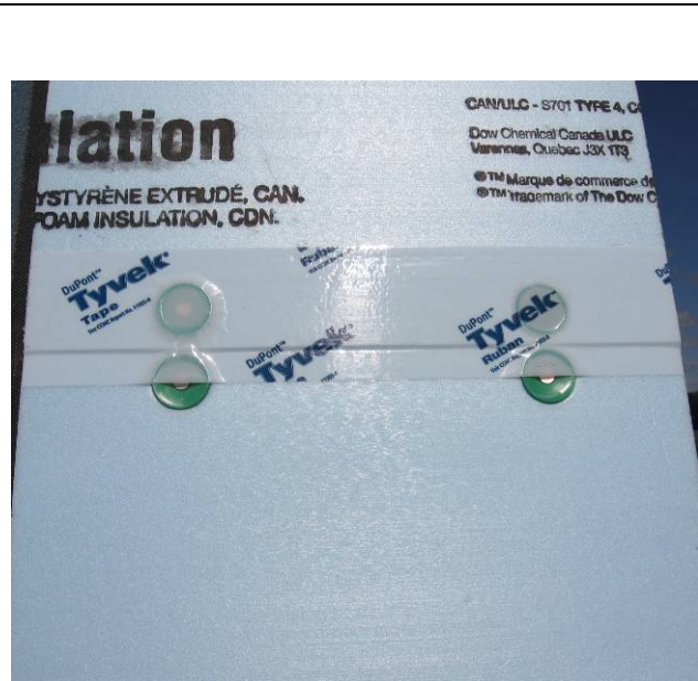
Figure 44. Dupont Tyvek tape on XPS—large sample
