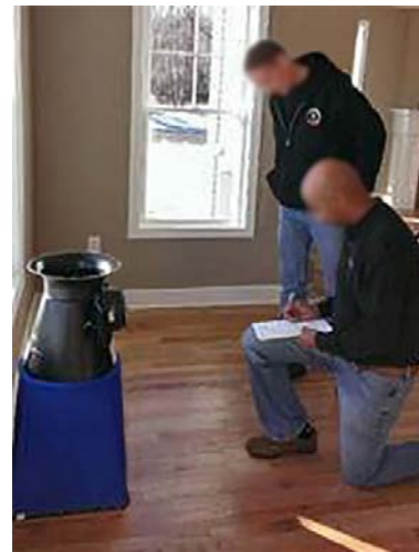
Figure 23. Measuring airflows with a low flow balometer
