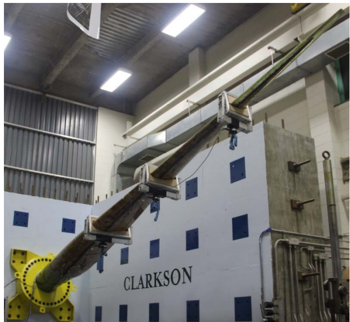
Figure 10. BSDS blade mounted for static testing.
