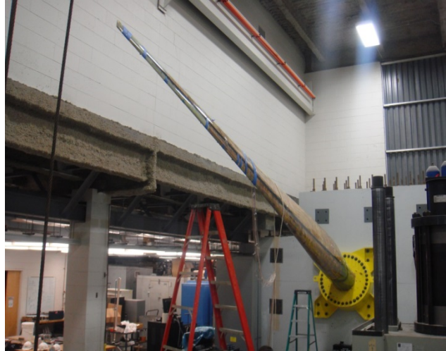
Figure 12. Experimental setup of the wall-mounted blade.
