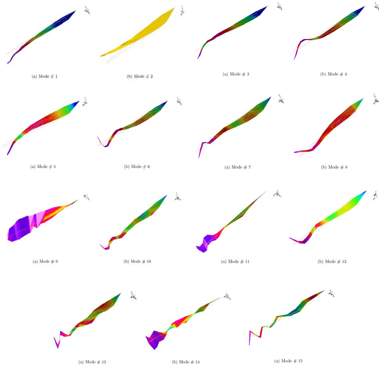
Figure 14. Normal modes estimated from the impact test for the wall-mounted blade.
