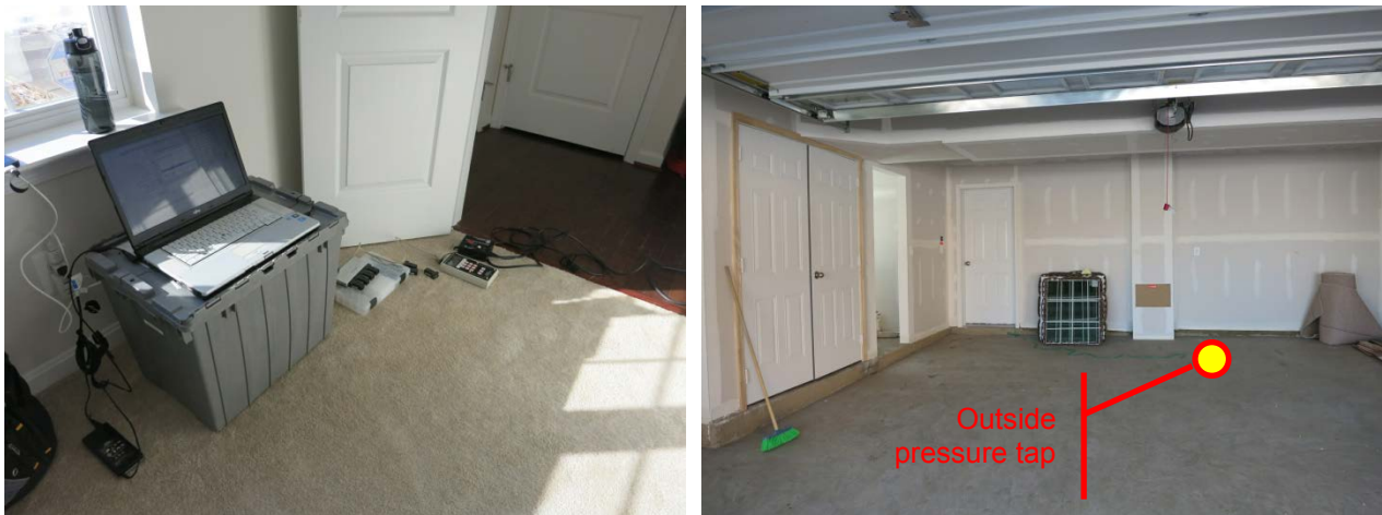
Figure 20. Multifan test setup, outside pressure tap in garage
