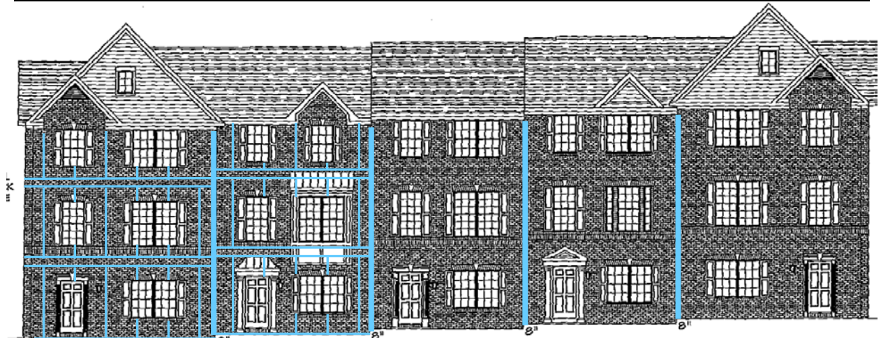
Figure 7. Experimental air barrier listing, with unit numbers and taping locations
