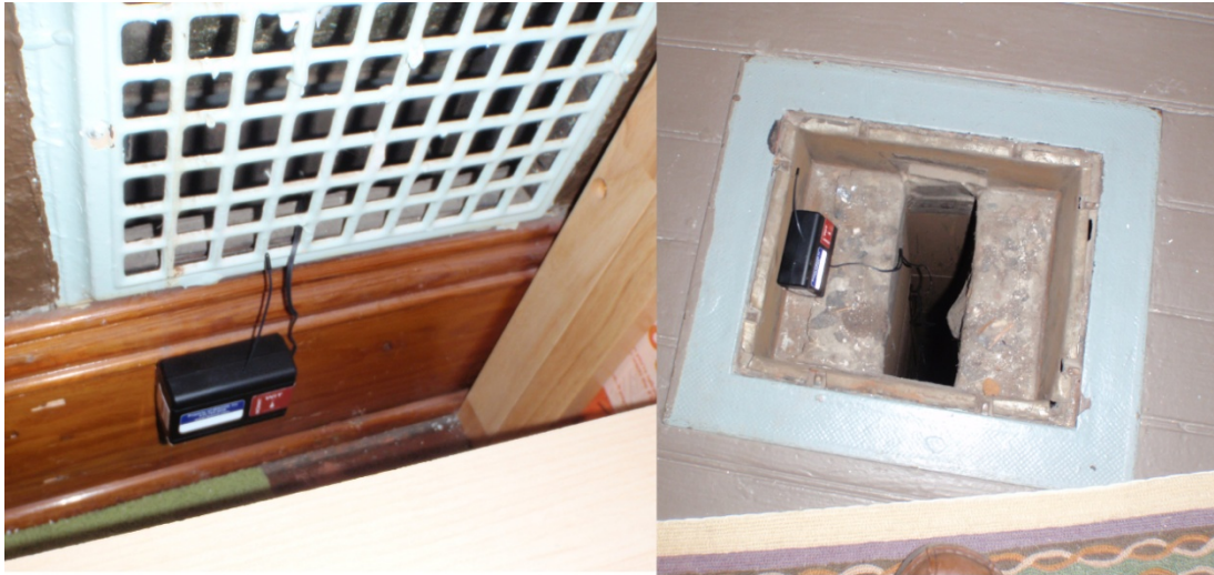
Figure 10. Temperature sensors at the register of the longest duct runs in Test House 2
