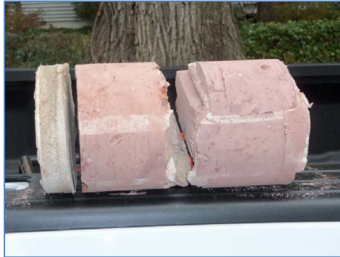
Figure 43. Core from B home for an exhaust fan
