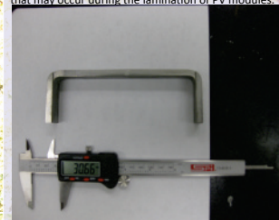
ABOVE: A leveling tool may be used to grade the sand substrate. In the example here, a “C” shaped object is used to flatten the sand. The tool shown is recessed (out of plane to the photo) in its center (between the handles at the edges). The tool shown will level the sand between the handles when dragged over the sand in the direction towards the top or bottom of the photo. In practice, any straight-edge (such as a blade, rigid applicator, ruler, roller, or similar object) may be used to grade the sand.
