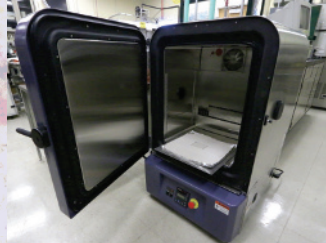
ABOVE: A circulating closed-loop controlled oven is required for the test. The differences in the duration and magnitude of radiation present are readily distinguished in the figure. If an aluminum foil substrate at least 300 mm x 300 mm in size is used, multiple specimens may be tested simultaneously in the oven. If space permits, sand used in subsequent tests may be equilibrated in the oven, e.g., in a jar or other container, while it is being used for the size change test.
