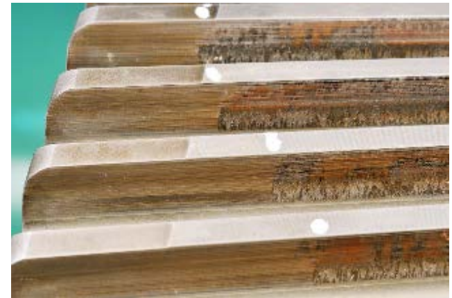
High-Speed Stage Gear Damage
