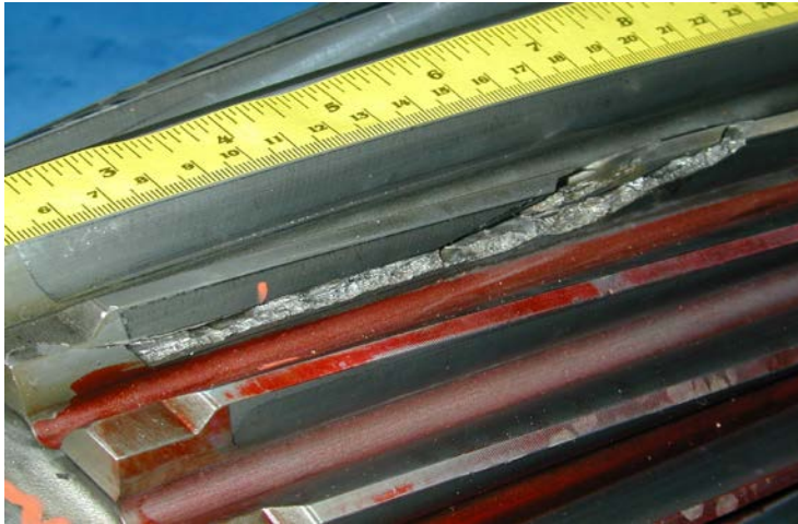
Bending Fatigue (intermediate-stage pinion)
